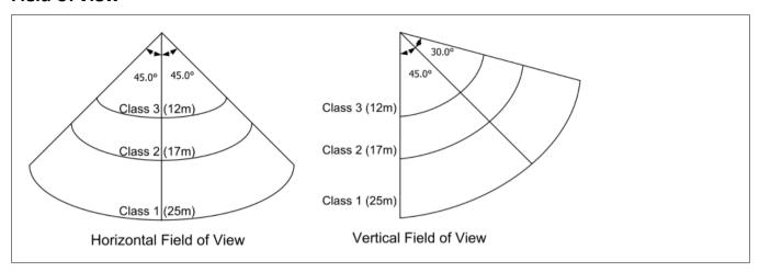
To comply with the directional dependence requirements for EN 54-10:2002 an angle of  $\pm 30^{\circ}$  from  $0^{\circ}$  ( $0^{\circ}$  = Orientation of detector in same axes as flame source) should not be exceeded, based on lab testing at a distance of approximately 5.0 ft (1.5 m).
